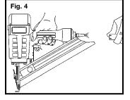
**9. DISCONNECT TOOL FROM AIR SUPPLY HOSE** before doing tool maintenance, clearing a jammed fastener, leaving work area, moving tool to another location, handing the tool to another person, or making adjustments. Fig. 4.
